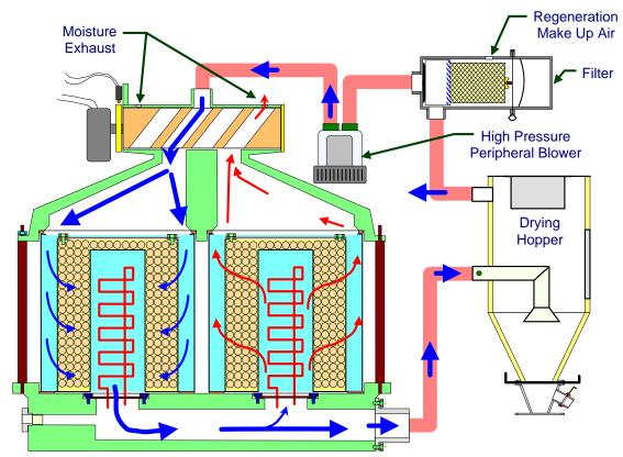
Figure 15: High Heat Model (180°F to 400°F) Air Flow Schematic
